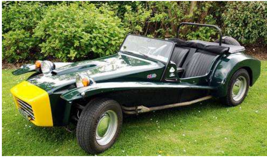
Figure 5: A later model right hand drive Ford 1600 GT crossflow powered S4 with the front indicator lights integrated with the front wings and a bonnet bulge to clear the downdraft Weber's air filter.
