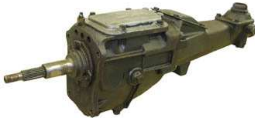
Figure 17: The Ford Mark 2 Cortina GT/Corsair 2000E (2821E) gearbox ( www.burtonpower.com ( http://www.burtonpower.com/ )).
