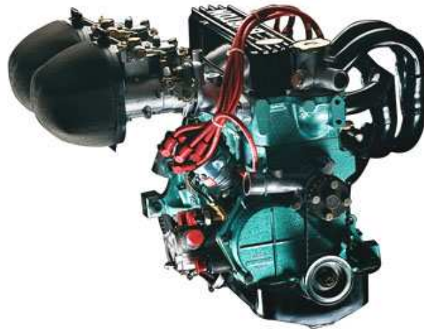
Figure 14: The Ford Kent 1600 cc crossflow engine ( www.burtonpower.com ( http://www.burtonpower.com/ )).
