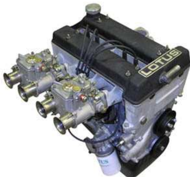
Figure 9: The 1558 cc Lotus Twin Cam engine as used in the Seven S3 SS, Seven S4, Elan, Elan +2, Europa Twin Cam, and Lotus Cortina ( www.burtonpower.com )
