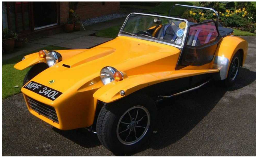
Figure 20: A later Twin Cam powered S4, fitted with the universal bonnet incorporating a bonnet bulge, showing the side screens with the sliding Perspex windows.
