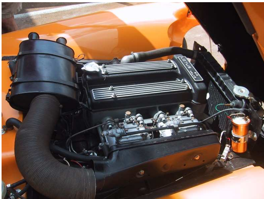
Figure 12: The engine bay of a Twin Cam powered Seven S4 showing the air box.
