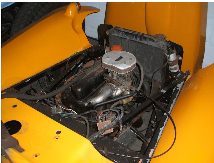
Figure 16: The engine bay of a 1600 cc crossflow powered Seven S4 showing the pancake air filter. This example is in need of restoration.
