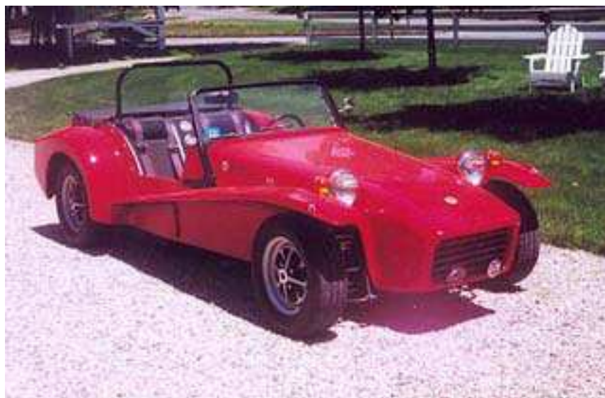
Figure 4: A later left hand drive S4 (designated by the front indicator lights integrated into the front wings) fitted with a Lotus Twin Cam as evidenced from the lack of a bonnet bulge. Unusually, the steel chassis side panels are body colored rather than being painted black.
